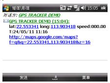
5.4.3. When lost fix to satellites, the message will includes the GPS coordinates of last known position and LAC code of current position as well.
