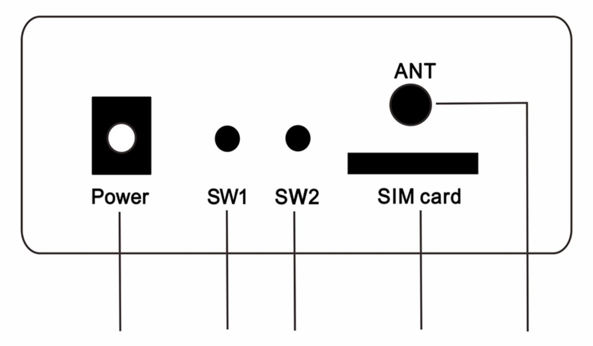
9-12VDC switch1 switch2 SIM card slot antenna
