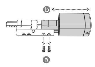
Adjust the length of the cylinder according to the door thickness, and then Fix with screws
