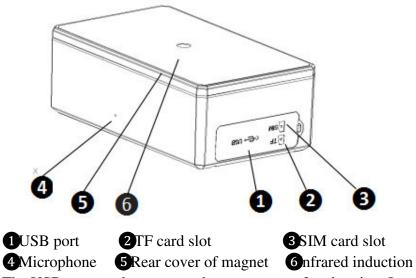
The USB port can be connected to a computer for charging. It can also be used for program upgrades.
