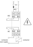
Do not apply voltage to terminals IN1 and IN2 - the control contacts must be potential-free!
